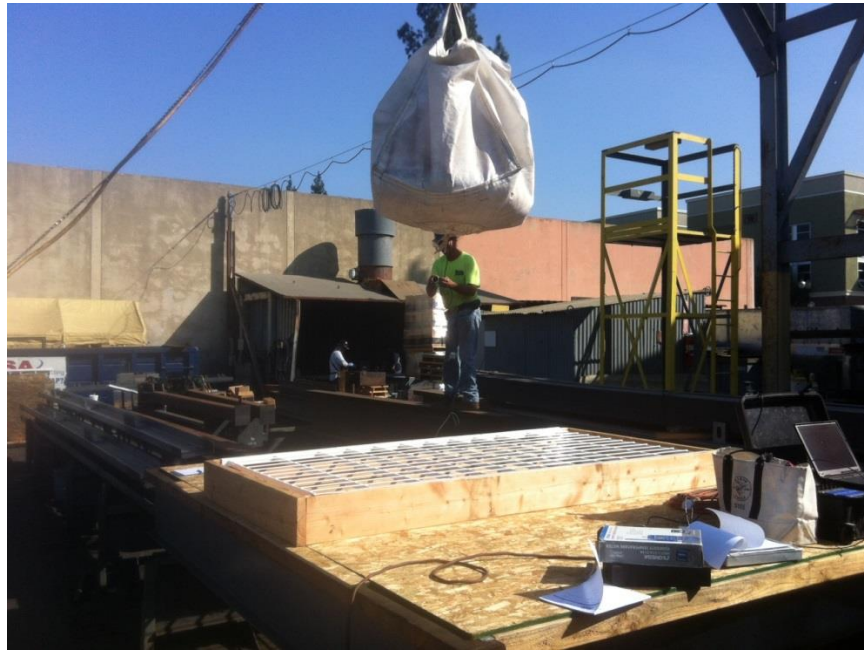
Photo No. 1 Test Specimen #1 prior to drop test
