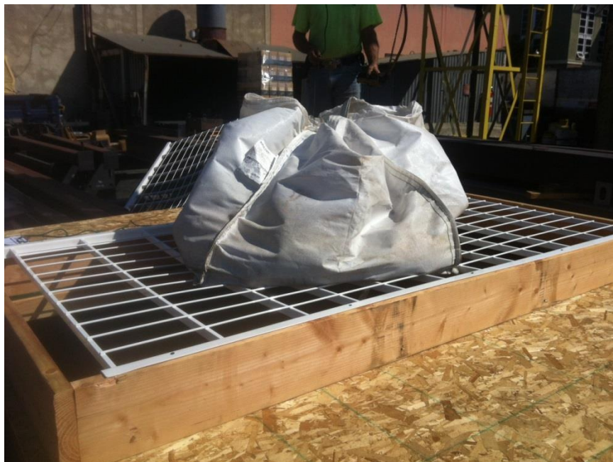
Photo No. 6 Test Specimen #2 after drop test
