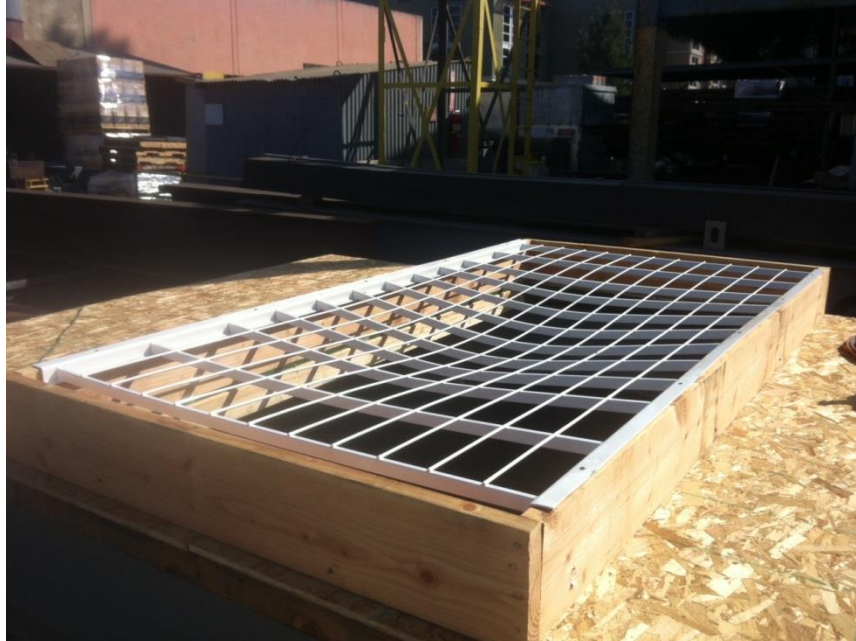
Photo No. 3 Test Specimen #1 deformation after drop test
