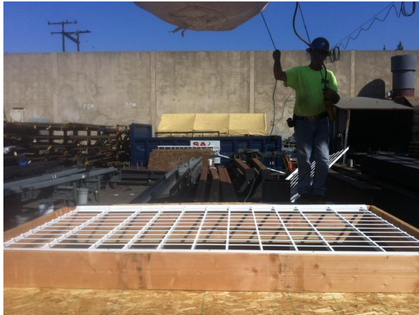
Photo No. 5 Test Specimen #2 prior to drop test
