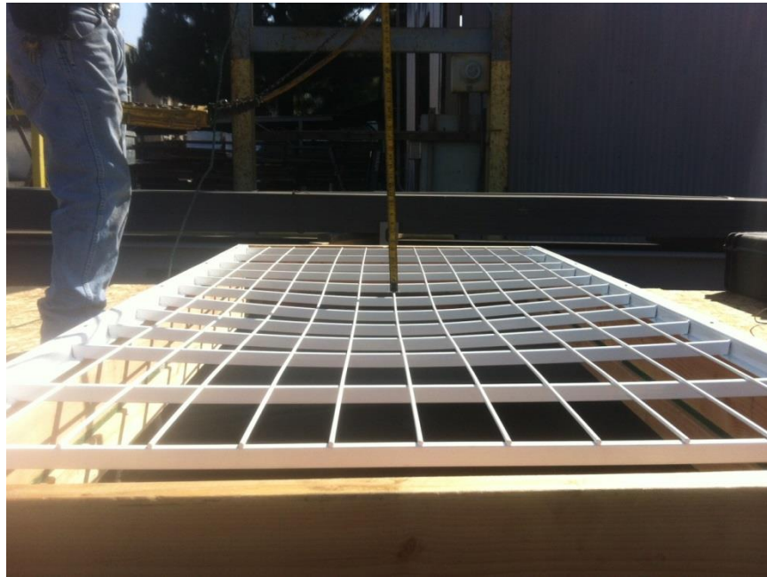
Photo No. 7 Test Specimen #2 deformation after drop test
